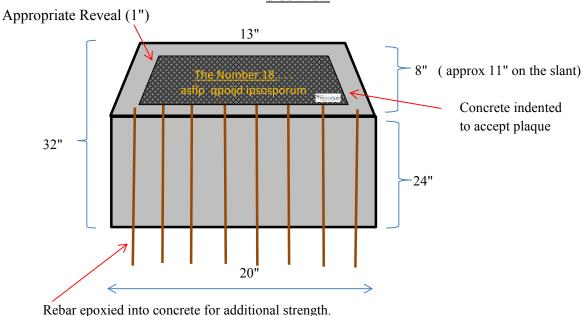
Concrete reinforced with rebar (size to be determined).
